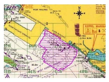
As per the project specifications Geometra's scope of work in the above project was to carry out bathymetric (Multi Beam Echo Sounder) monitoring interim survey in the designated areas on three monthly recurring basis. The purpose of the survey is to monitor the progress of reclamation work.
