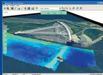
QPS was the first company introducing the "delta heave" method, which means that the quality of the final DTM is no longer affected by heave drift caused by vessel turns.
