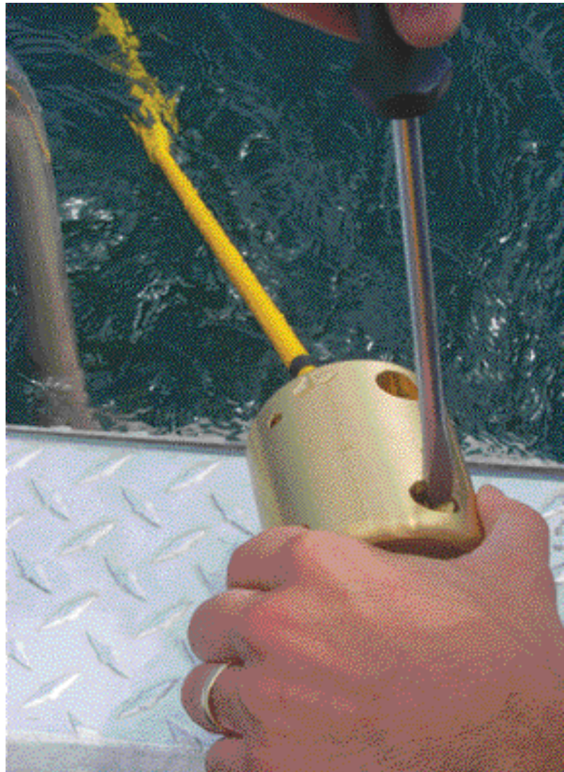
Brass tow cable weight attached to MMC's cable
