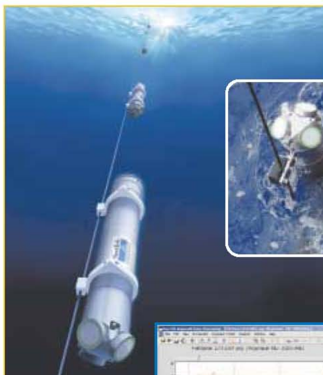
Typical deep-ocean deployment clamped directly to a mooring line.
