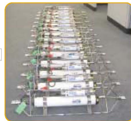
Multiple Argonaut-MD systems with integrated CT sensors and load cages
